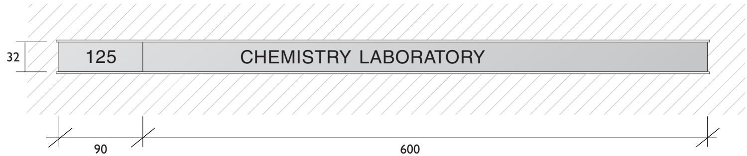
Sign specification as Type 2a
