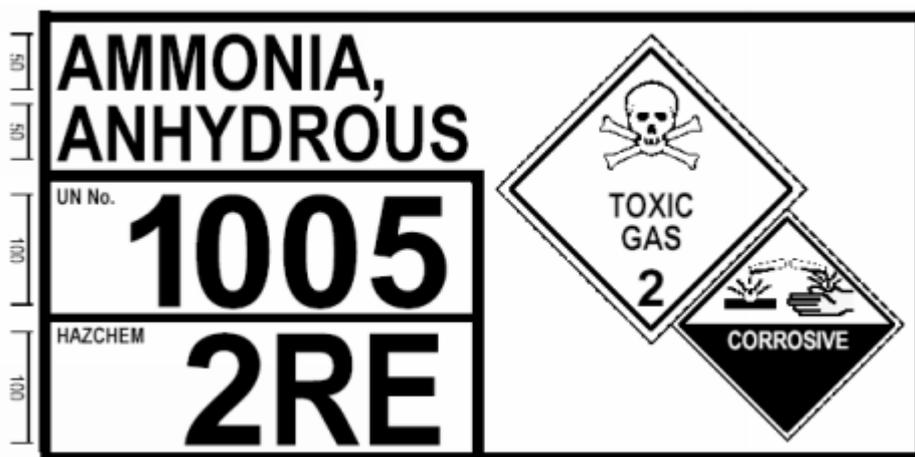
**Figure 4** Example a placard for bulk dangerous goods
